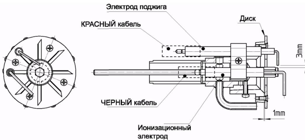
**УСТАНОВКА ЭЛЕКТРОДОВ ДЛЯ ГОРЕЛКИ GAMMA GAS X4 CE**
